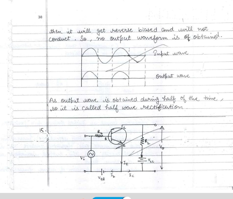
The transistor will work as an amplifier when Vo > Vi i.e. in active region when emitter-base junction is forward biased and collector output is reverse biased. i) Paramagnetic Substance ii) Diamagnetic Substance
